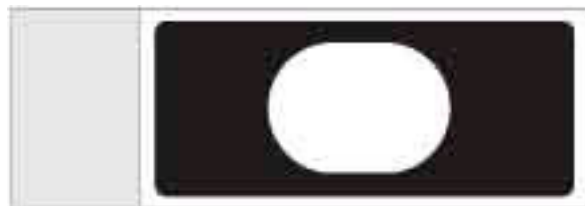
Figure 80 Standard 25 mm x 75 mm x 1 mm slide used during the manufacturing of 17 x 24 mm oblong, single well fluorescent particle slides.
