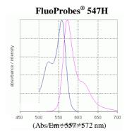
The FluoProbes® 547H is compatible with **orange standard filters.** It is **photostable**, pH independent and **hydrophilic** for a lower background.
