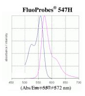
The FluoProbes® 547H is compatible with **orange standard filters for fluorescein.** It is **photostable**, pH independent and **hydrophilic** for a lower background.
