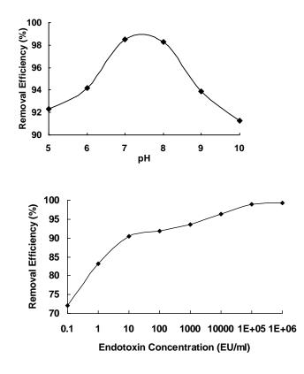
The Effect of pH on Removal Efficiency
