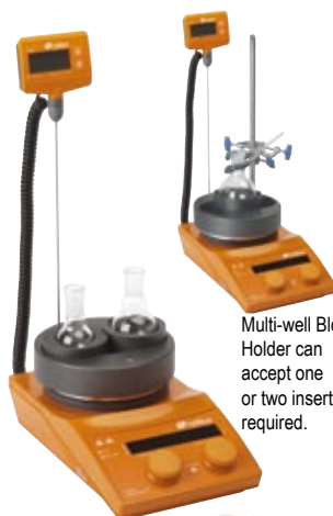
Multi-well flask inserts are available for 10ml, 25ml, 50ml, 100ml & 150ml flasks
