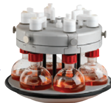
Carousel 6 locates on to the Storm without tools
