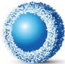
1000 Å 2.7 micron particle
