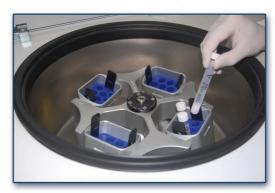
Centrifuge at high speed (≈2500 rpm) for 5 minutes.
