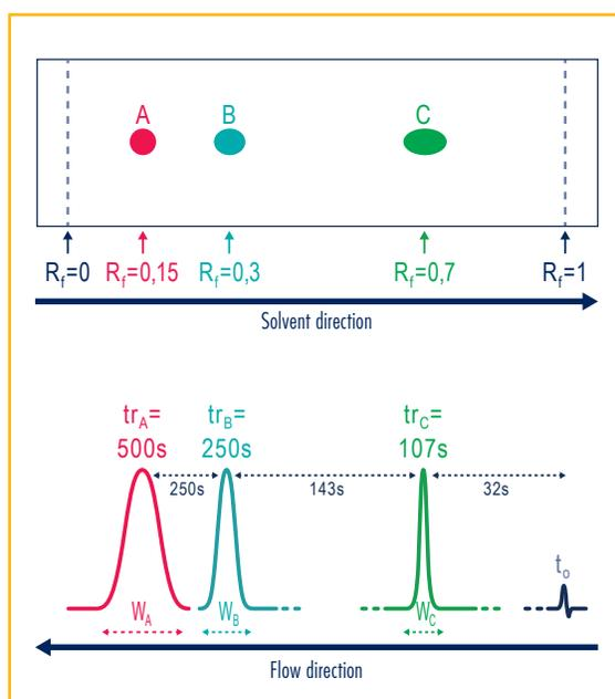
The  $\Delta R_f$  (frontal ratio) optimization allows the best transposition on the Flash/Prep column.
