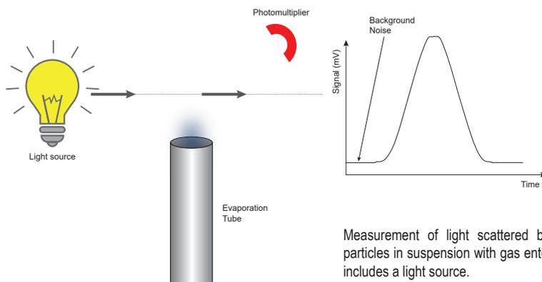
Measurement of light scattered by a stream of solid particles in suspension with gas entering a flow cell which includes a light source.
