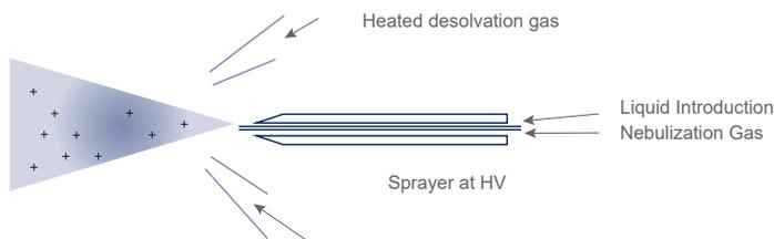
Electrospray is produced by applying a strong electric field to a liquid passing through a capillary electric field to a liquid passing through a capillary tube with a weak flux.
