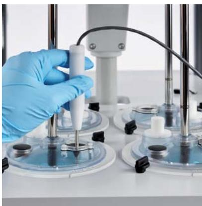
Manual temperature measurement using 708-DS temperature probe
