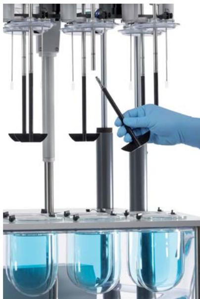
Upper shaft receptor and lower paddle piece
