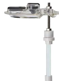
Float-A-Lyzer with holder and evaporation cover
