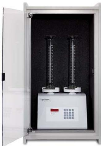
350 Tapped Density Tester, dual-platform in the specially designed acoustic cabinet
