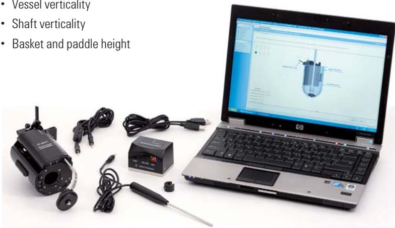
Agilent 280-DS Mechanical Qualification System and Workstation Software
