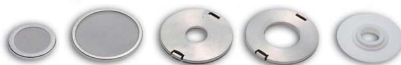
(Left to right) Paddle Over Disk assemblies, transdermal patch holders and suspension cup
