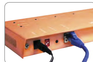
Power and Ethernet Connection
