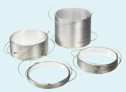
FlowSyn coil reactors consist of 1mm id tubing wound around an aluminium 'mandrel'. They have been designed to allow you to rapidly switch between different sizes and materials for different reactions, making FlowSyn an ideal research tool.
