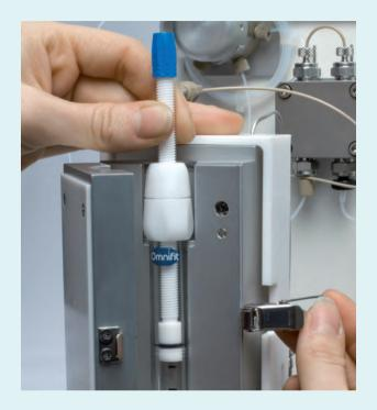
Adjustable column for varying reaction scale
