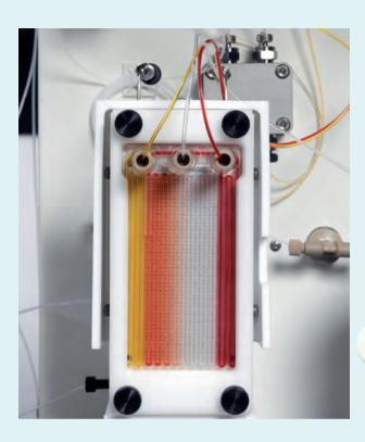
Fast, turbulent mixing in 1 mm id channels
