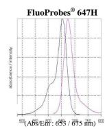
The FluoProbes® 647H is compatible with **far red standard filters.** It is **photostable**, pH independent and **hydrophilic** for a lower background.
