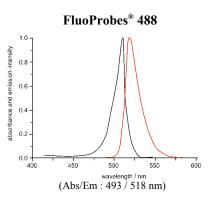
The FluoProbes® 488 is compatible with **standard filters for fluorescein**. It is **photostable**, pH independent and **hydrophilic** for a lower background.
