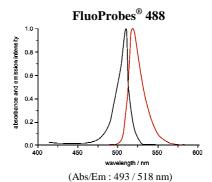
The FluoProbes® 488 is compatible with standard filters for fluorescein. It is photostable, pH independent and hydrophilic for a lower background.
