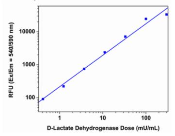
**Figure 1.** D-LDH dose response was measured with Amplite<sup>™</sup> Fluorimetric D-LDH Assay Kit in a 96-well black plate using a Gemini (Molecular Devices) microplate reader. As low as 1mU/mL D-LDH in 100 µL volume can be detected with 30min incubation.
