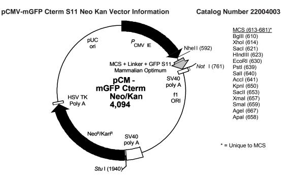
Figure 2. Feature Map of pCMV-mGFP Cterm S11 Neo Kan. Unique restriction sites shown flanking key modules. The Not I site follows the mGFP S11 stop codon. Genes are cloned with initiator codons just after Nhe I in the multiple cloning site (MCS) and in-frame with the downstream linker and GFP S11 module. The structure of expressed proteins of interest (POI) is POI-linker-GFP S11.
