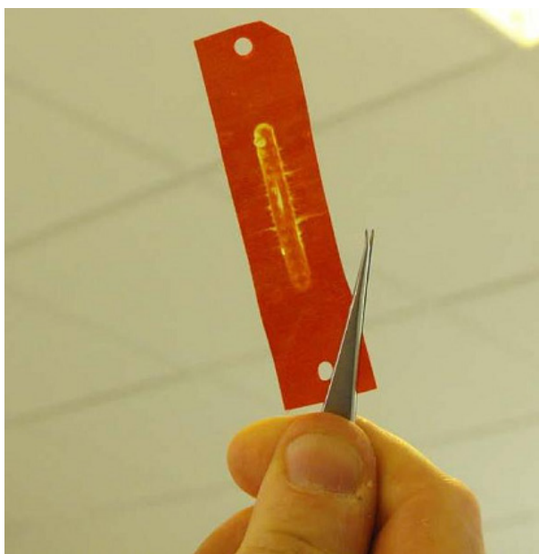
Fig 7. Deterioration of KOBRA® CELL Membrane
