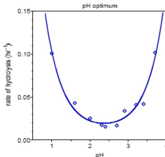
Figure 4. The optimum stability of the epicocconone adduct is achieved at about pH 2.4. Fitting the data to a general acid/base mechanism gave a pseudo-first order rate constant of  $k_B' = 1.03 \times 10^5 \text{ s}^{-1}$
