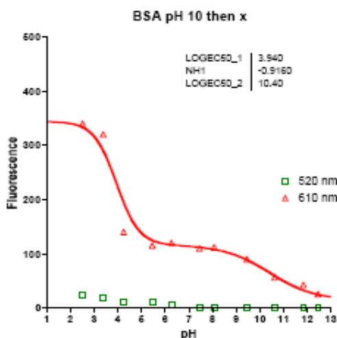
Figure 3. Fluorescence of epicocconone in the presence of protein (BSA) at varying pH. The red trace shows emission at 610 nm and the green squares are emission at 520 nm.
