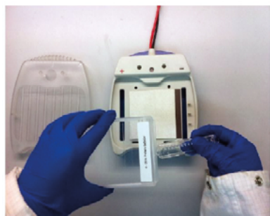
Picture 1: Opening the cassette with the comb
