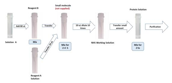
Scheme 1. Schematic diagram of the work flow for preparing BSA-small molecule conjugates
