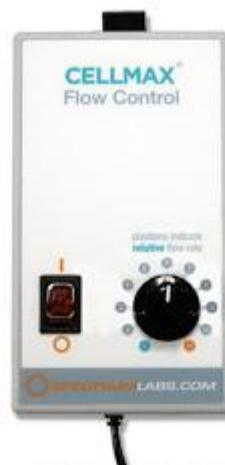
A detachable power cord links the pump base to a peripheral Electronic Control Unit (ECU). The ECU has a magnetized rear surface for easy attachment to the outside surface of an incubator. The ECU contains an 11 position variable speed potentiometer for flow rate control.
