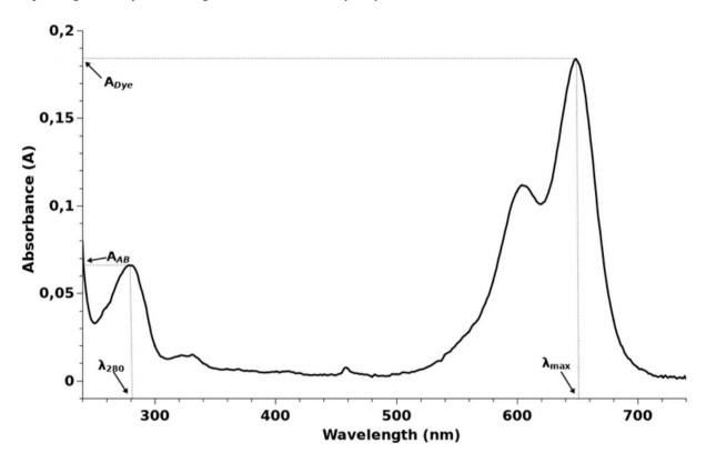
An absorption spectrum of a labeled antibody contains dye peak (with longer wavelength), and antibody peak (at around 280 nm). Dye to antibody ratio is calculated using the following formula:
