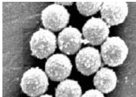
Figure 1 SEM Photo of Spherotech Cat. No. CM-30-10 (Carboxyl Magnetic Particles, 2.5% w/v, 3.36µm, 10 mL). at 5000x.
