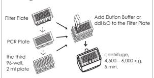
Add Elution Buffer or ddH2O to the Filter Plate. Stand for 3 min. Apply vacuum to elute DNA.
