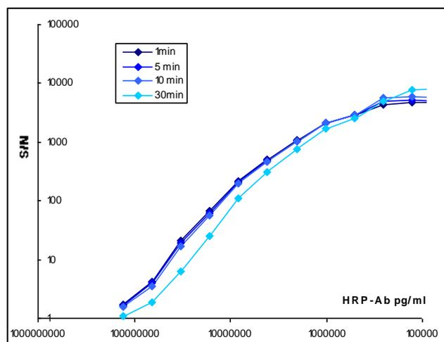
Figure B: Photostability of light emission with UptiLight™US ELISA HRP Substrate. Luminescence was recorded with 0.1sec integration time after a 1, 5, 10 or 30min pre-incubation period.
