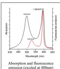
emission (excited at 488nm) spectra of JC-1 in pH 8.2 buffer containing 1 % (v/v) DMSO.
