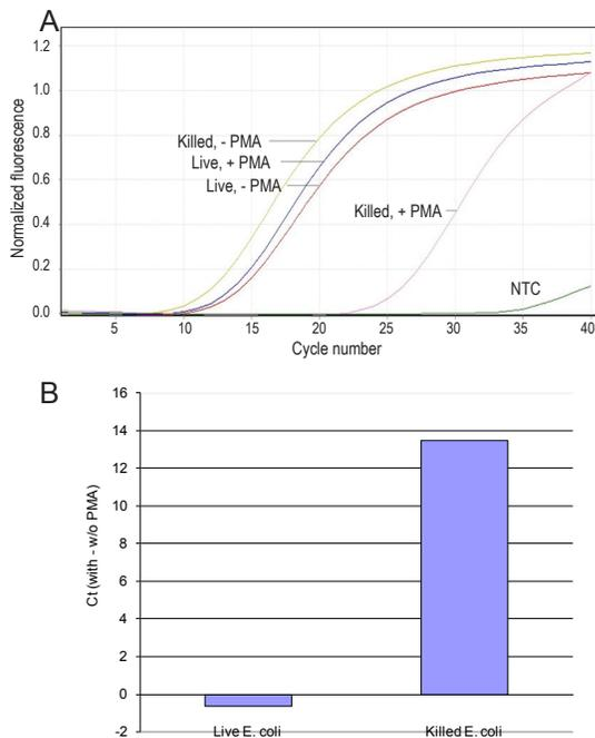
Figure 4: Effect of PMA on qPCR of DNA from live and heat-treated *E. coli*. qPCR was performed using primers against a region of the 16S rRNA gene. (A) Representative amplification curves for real-time PCR performed on DNA from PMA-treated live and heat-killed *E. coli*. (B) The Delta Ct of live and killed *E. coli* with and without PMA treatment. The Ct value of sample without PMA was subtracted from the corresponding sample with PMA cross-linking (Ct with PMA – Ct without PMA).
