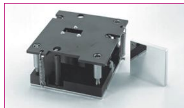
Relative Specular Reflectance Accessory, 6°
