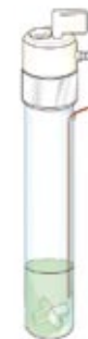
Flexible wire Probe inserted via a glass pocket in the RR98051 Reaction Tube
