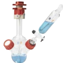
100ml vessels with two sidearms, baffles, dropping funnel and stirrer seal
