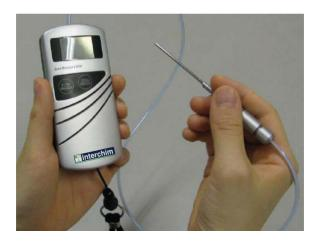
**Interchim' Gas Leak Detector** adapts thermal conductivity technique between target gases and referential gas.
